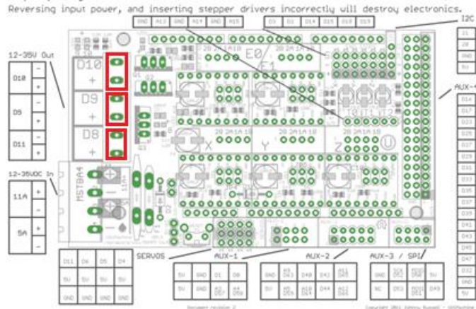
From top to bottom: extruder heater 1, fan, and heated bed heater.
