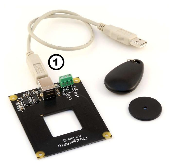
1. Connect the PhidgetRFID board to the computer using the USB cable.
