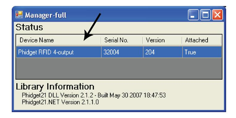
Run the program *Manager-full* to make sure that the *PhidgetRFID* is properly connected to your PC.
